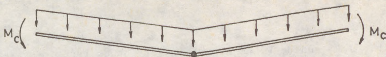
Figure 7 - Reduction to zero of the beam stiffness after the formation of a hinge at mid-span.
