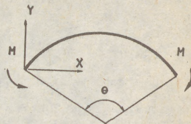
Fig.4 Circular arch in uniform bending
